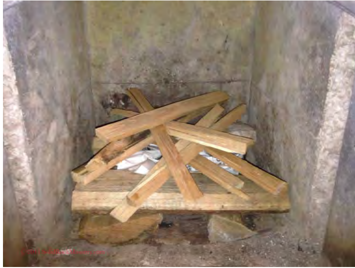
Fires 12-13: approximately 25 lb of wood, spaced every 8 hours.
