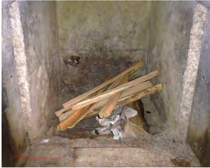
Fires 1-3: approximately 5 lb of wood, spaced every 8 hours.
