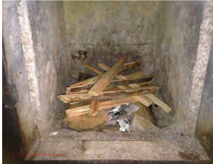
Fires 7-9: approximately 15 lb of wood, spaced every 8 hours.
