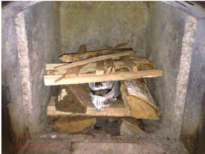
Fires 10-11: approximately 20 lb of wood, spaced every 8 hours.
