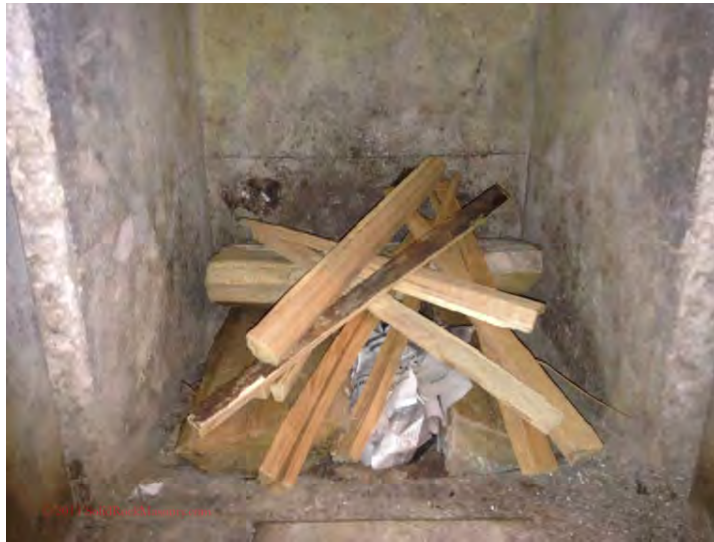
Fires 4-6: approximately 10 lb of wood, spaced every 8 hours.
